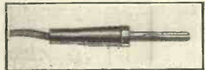
Fig. 4.—One of the terminal pins of the coils.
